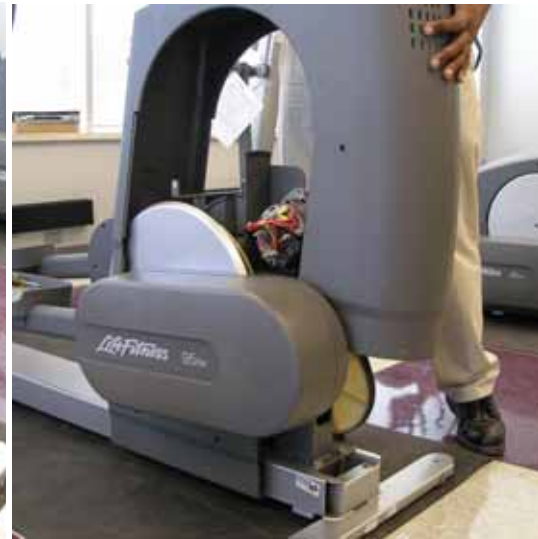
Fig. 2: removing the main shroud
